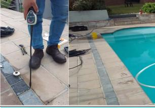
Area where tracer gas was detected and leak is suspected to be
