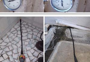
Tracer gas detected in the shower and on the exterior wall of the shower.
